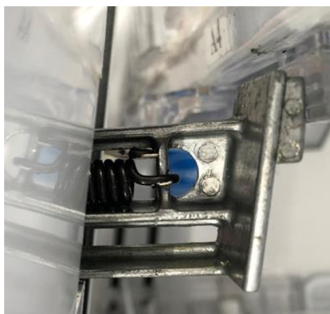
Cup Picker/Plunger shown in the Out position.
